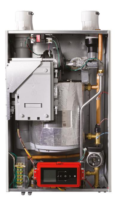
CTRLMAX Control System -EZ Setup allows for quick 60 second setup. Easy troubleshooting in plain text, no codes. Stainless Fire Tube Heat Exchanger. 3 in 1 Universal vent adapter directly accepts PVC. Large plate heat exchanger provides industry leading performance. 5+ GPM hot water while fully condensing in DHW mode.
